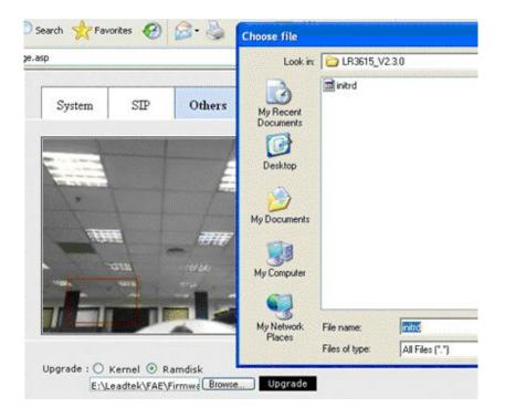
3) A message box pops up and a down counter shows the remaining time left of the whole upgrade procedure. The surveillance camera will reboot itself automatically when the upgrade procedure is done.
